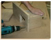
Drill and countersink the 'tunnel' to front of 'house' and secure with screws.
